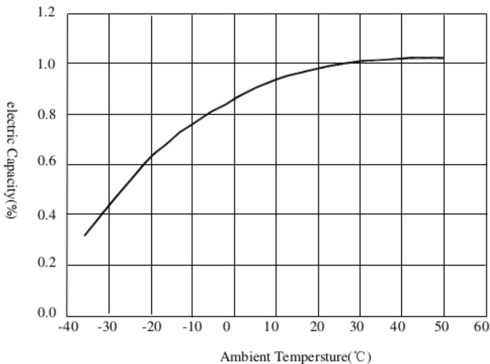
As represented by the graph above, the capacity of the battery will decrease when the temperature is too low. For example, if the temperature decreases by 20°C, the
